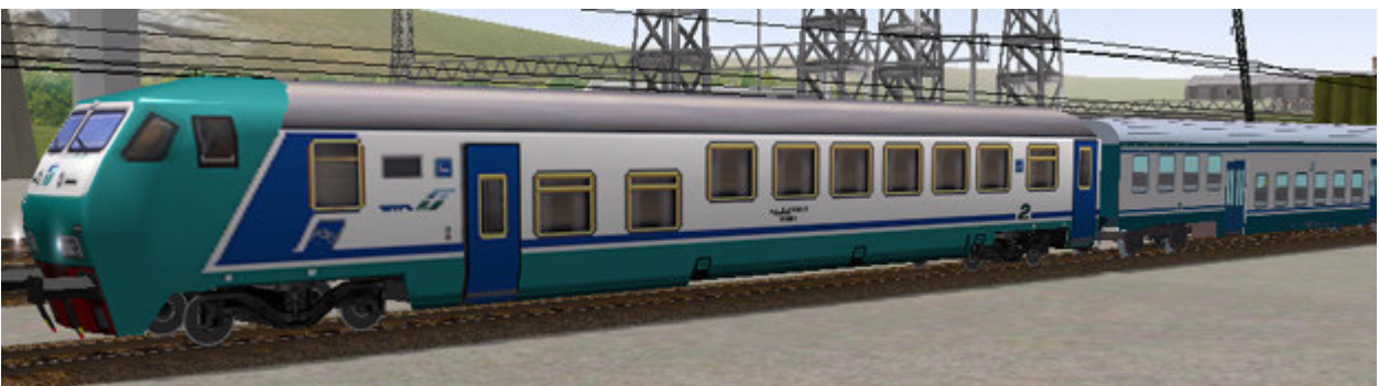
UIC-X Coach transformed into a Driving cab, with entrance for disabled, with Low floor stock, Torino 2000. Model Pek.
