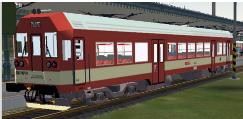
A Diesel electric motor car, compared to the 842, which has a hydraulic drive. There is a matching trailer Class 943.
