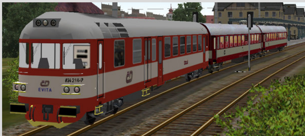
DMU motorcars for fast regional trains. The opposite end to the picture has a corridor entrance through the driver's cabs. The 852-4 pull a standard type Btn passenger cars, which are equipped with their own passenger heating.
