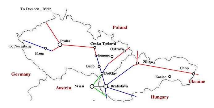
A highly schematic map showing the Trans European Network (TEN) corridors going through Czechia and Slovakia Blue is electrified at 25kV 25Hz AC, Red 3000 V DC. Green is 15kV AC 16.7 Hz.
