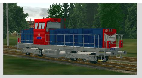
The 714 are 29 Locomotives rebuilt from retired class 735 with new Skoda motors (Some are 600kw and 90 km/h). The 714.2 have a lighter axel load. Both have electronic braking
