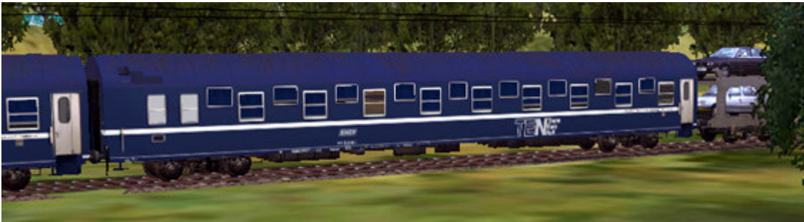
A T2 sleeping car, showing the windows for the twin level compartments. Model Sylium (payware). No model of the MU available.
